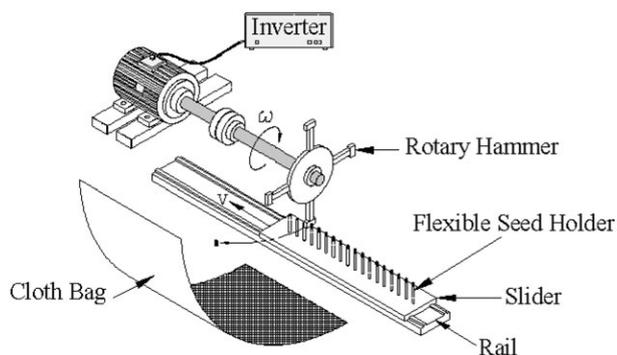
**Figure 2** Diagram of the impact damage assessment device.
