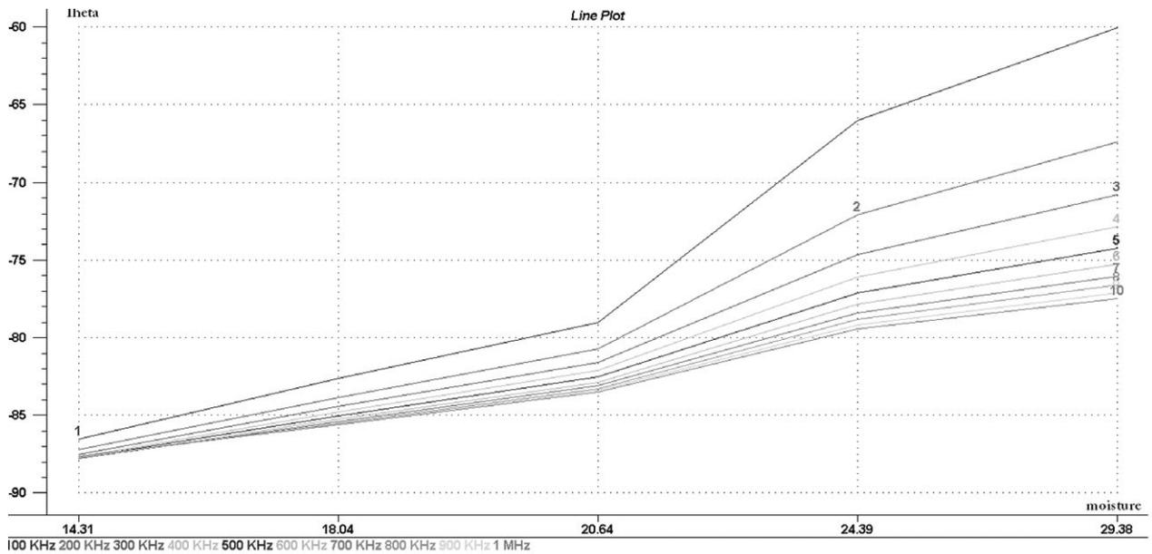
Figure 3 Moisture dependence of the Theta of wheat grains at 100–1000 kHz frequency.
