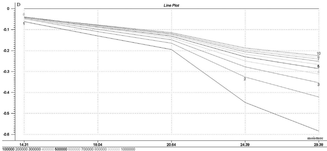
Figure 4 Moisture dependence of the impedance of wheat grains at 100–1000 kHz.
