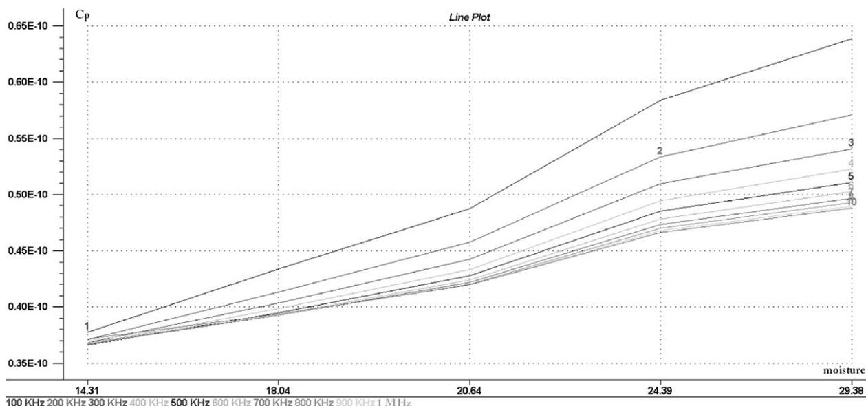
**Figure 1** Moisture dependence of the capacitance of wheat grains at 100–1000 kHz frequency.
