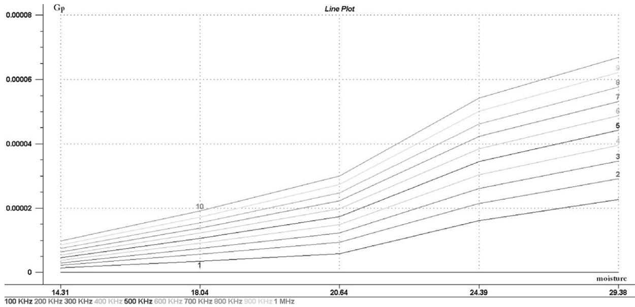
Figure 2 Moisture dependence of the conductance of wheat grains at 100–1000 kHz frequency.
