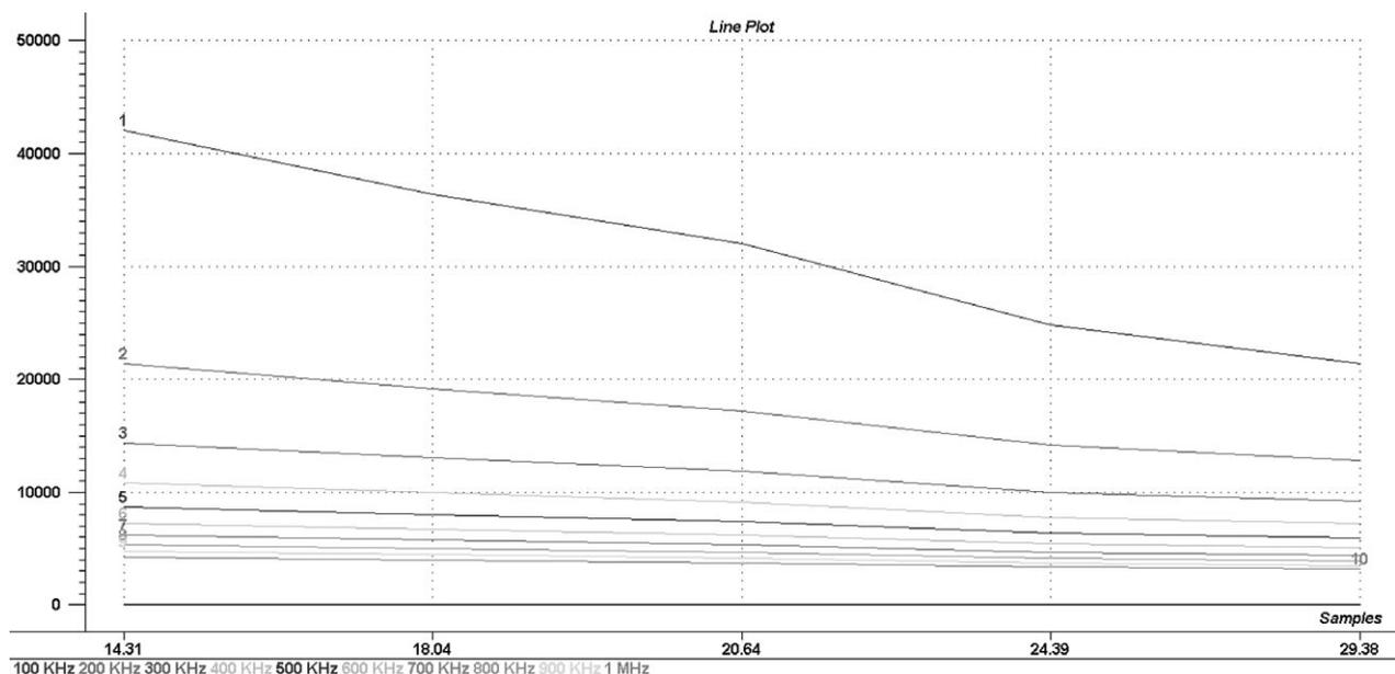
Figure 5 Moisture dependence of the dissipation of wheat grains at 100–1000 kHz.
