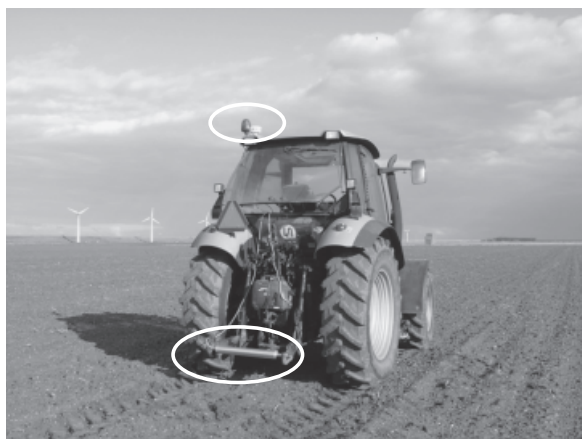
Figure 4 Field measurement with \gamma ray soil sensor.
